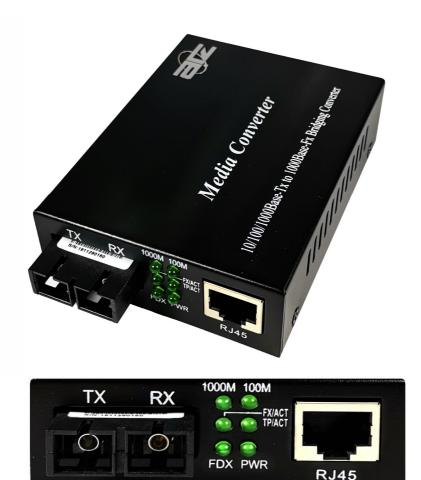
This ATZ FO-MC-GE-MMDP0.55K-SC 10/100/1000M Ethernet media converter adopts switching technology to fulfil media conversion. It complies with IEEE802.3z and IEEE802.3ab standards, and supports two types of media network connections: 10/100/1000Base-T and 1000Base-SX/LX. It inter-converts electrical signals of 10/100/1000Base-T twisted pairs with optical signals of 1000Base-SX. It extends the network transmission distance to 550m via multi-mode fiber cable OM1 / OM2.
