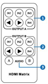
1 IN1/IN2/IN3/IN4: Selects the OUTPUT A port input channel, corresponding on-panel light is on.
