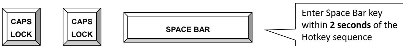
**Example 2** – To switch to Bank 1 Port 1, press **Caps Lock + Caps Lock and 1 + 0 + 1**
