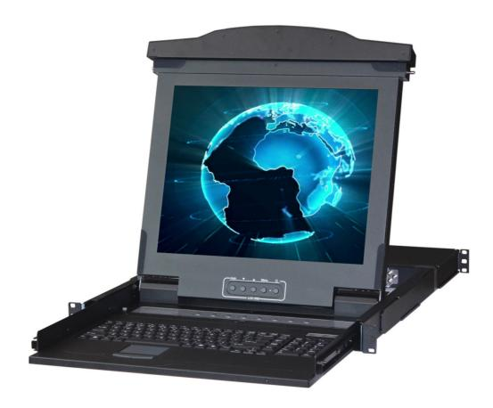
ATZ range of LCD console drawers provides a variety of features that simplify to access servers to making system monitoring, troubleshooting and software upgrades.
