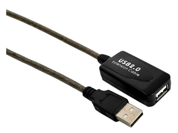
USB 2.0 A-Male to A-Female Active Extension Cable 15m is a bus-powered extension cable that can be used to increase the distance of a device without the worry of signal loss and potential performance problems. It contains active electronics which boost the USB signal for maximum reliability and performance over extended distances. It's plug-and-play with no additional drivers required. It support Win, Mac, Linux OS
