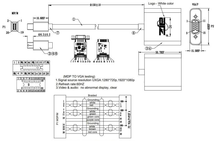
Remark: 13&14 are grounding, PINs could be disconnected.
