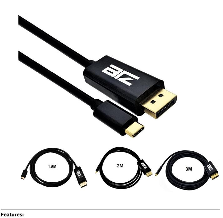
USB TYPE C (Thunderbolt 3 Port Compatible) to DisplayPort cable connects a Computer with a USB Type-C port to a monitor or projector with DisplayPort input; USB-C port of host requires DisplayPort Alternate Mode support to view video over USB.
