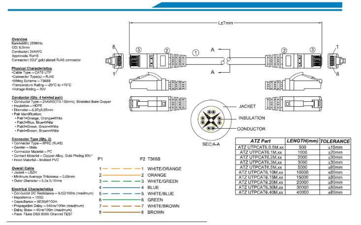
Cat.6 fixed length network patch cords are the perfect combination of value and performance. Available in a large assortment of colors and lengths, we have a cable to fit every situation. Each cable is made of 24AWG, pure copper listed pair conduits with 50-micron gold plated contacts, snagless design(which avoids tangles), with strain relief boots.
