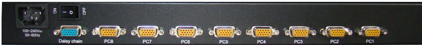
8 port LCD Drawer Rear VIEW
