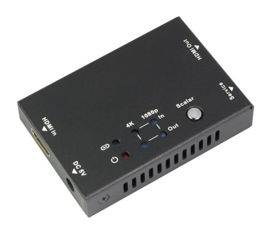
The machine is a HDMI Repeater with one input and one output port, it can do scaler up/down/pass-through . Furthermore, both input and output HDMI support video resolution up to 4K2K@60Hz (YUV444) and HDMI high resolution digital audio formats bypass, LPCM 2CH, Dolby TrueHD, Dolby Digital Plus, Dolby Atmos and DTS-HD Master Audio, audio sampling rate up to 192 kHz. HDCP 2.2 and CEC bypass supported.
