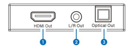
**HDMI Out:** Connect to HDMI display devices such as TV/Projector.
