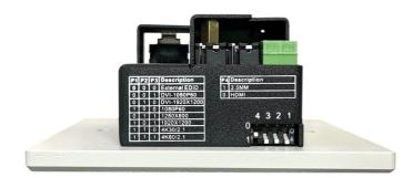
When using the internal EDID, plug the HDMI cable of the display into the input port, then select code to 000, wait for 2 seconds then connect normally.
