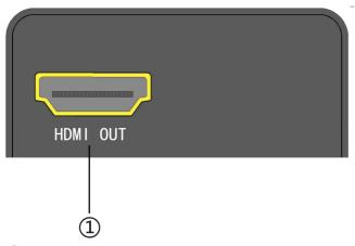
(1) **HDMI OUT:** HDMI output interface. (Connect to display devices, such as TV, monitor, projector.)
