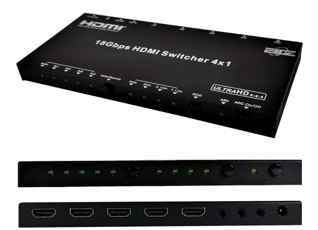
This is a high performance HDMI 4x1 switcher that supports HDTV formats up to 4Kx2K@60Hz and all HDMI 3D TV formats. It can extract HDMI stream audio to separate digital and analog audio output. This product supports HDCP repeater/CEC/ARC functions. Select any of the inputs by front panel button or IR Remote, the corresponding indicator LED on the front panel will be illuminated.
