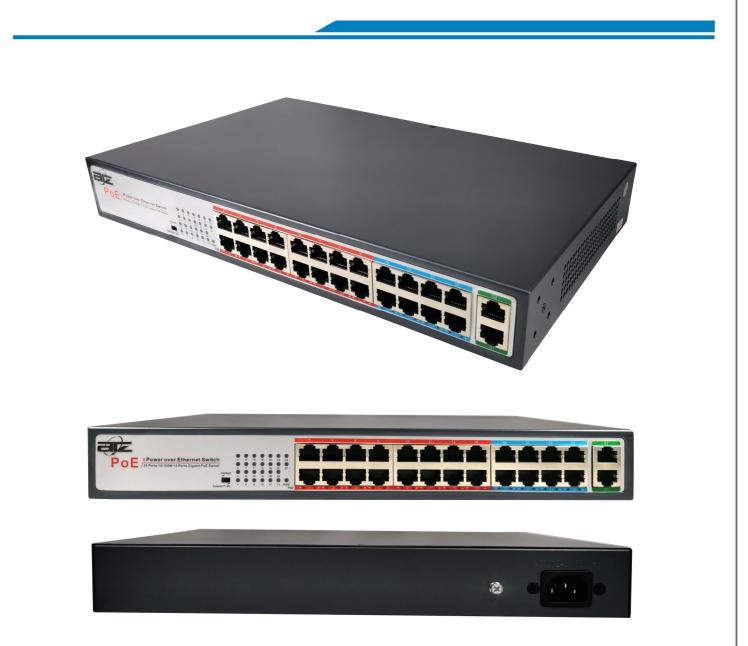
ATZ POE-SW24PL is an unmanaged PoE switch. It has 24\*10/100M PoE ports and 2\*10/100/1000M uplink RJ45 ports . Port 1-24 can support IEEE 802.3af/at standard PoE power supply, and single port PoE power reaches 30W. The maximum PoE output power is 250W. As a PoE power supply device, it can automatically detect and recognize the power receiving equipment that meets the standard and supply power through the
