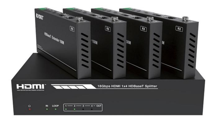
This 18Gbps HDMI 1x4 HDBaseT Splitter can distribute 1 source signal to any 4 display devices. Support video resolution up to 4K2K@60Hz 4:4:4. It is designed with 1 HDMI loop output and 4 HDBaseT outputs. The HDMI signal transmission distance can be extended up to 120 meters at the resolution of 4K2K@60Hz, or 150 meters at 1080P@60Hz via a single CAT6/ 6a/7 cable. The product supports IR and RS-232 signal pass-through, audio extract function and advanced EDID management.
