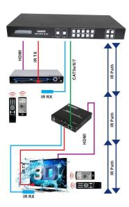
The matrix is not only a switcher and extender of multiple HDMI signals to multiple HDMI receivers located remotely, it also passes IR control signals through the IR call-back system to the matrix and HDMI sources for full, independent control of all connected inputs from output locations.
