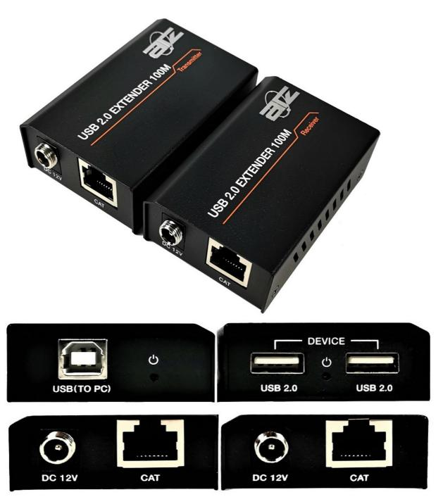
The USB 2.0 Extender can extend USB signal up to 100 meters / 328ft via Cat 5e/6 cable. In transmitter, the USB-B port is connected a PC. In receiver, you can connect a device with USB port at the two USB ports such as U disk or printer, etc. Transmitter and Receiver support PoC (Power over Cable) function. The product can be widely used long distance signal transmission between a PC and USB device. Simple plug and play, no drive and setting installation required.
