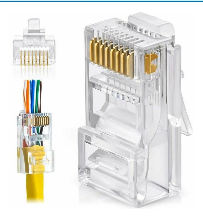
This Cat.6 RJ45 Unshielded plug features a Pass-Through open-end design. Feed the wires through the connectors and crimp with the appropriate crimping tool. Do not need to measure the length of the outer jacket to strip.
