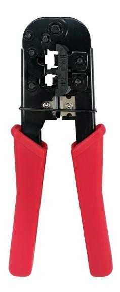
This 3-in-1 crimping tool cuts, strips, and crimps, providing a reliable & robust crimp installation for voice and data applications for Cat5/5e/6 - 8P8C/RJ45, 6P6C/RJ12, 6P4C/RJ11, 4P4C & 4P2C connector plugs. The tool has a built-in wire cutter and stripper and is manufactured from durable steel with soft cushioned grips.
