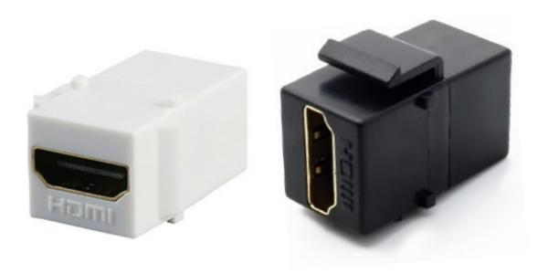
This is a sturdy HDMI keystone coupler that will snap into any standard keystone wall plate or patch panel, providing a secure, and vertically oriented HDMI female to female pass-through solution for all AV configurations for home or commercial applications. Supports 3D, 4K, Audio Return Channel, CEC, and Ethernet features of your HDMI cables and devices without any signal loss.
