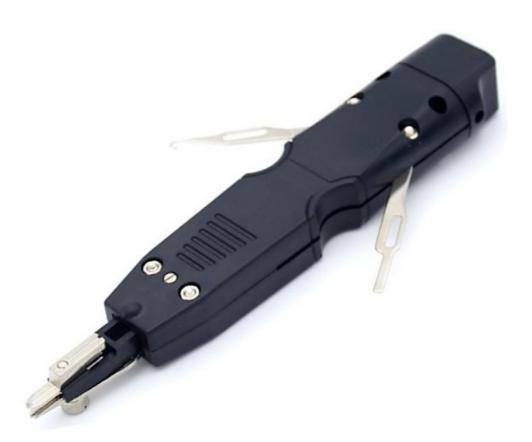
Multifunctional tool used for Industry standards Krone 110 Style Impact Punch Down & 10 pairs Module (Pouyet Type). Hook and Spudger tools are built into the handle. All blades are interchangeable and reversible with cuts function on one end, blade is easy to xchange.Specially-made tool head for durability.
