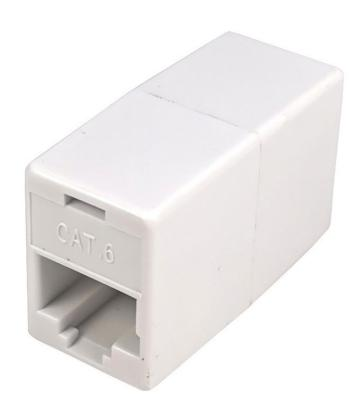
This in-line coupler provides a female-to-female feed-through connection for easy cable hook-up. The 1-1 wiring configuration is compatible with both T568A and T568B wiring schemes. For use with Cat 6 Ethernet cables and connectors one RJ-45 female to one RJ-45 female. Type 8 conductor straight-thru RJ-45 Cat 6 and designed for computer networking applications.
