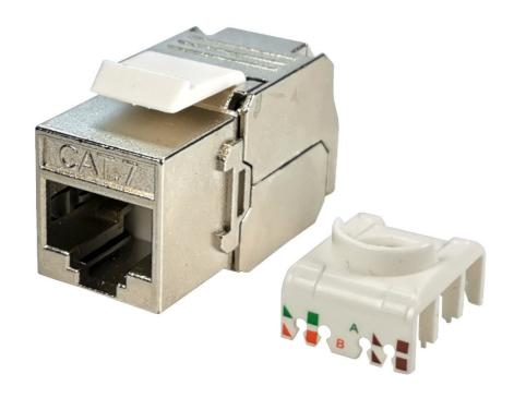
Cat 7 Shielded Keystone Jacks are the perfect choice for a complete Cat 7 shielded 10 Gigabit network system. This Cat 7 keystone jack fits patch panels or wall plates with standard keystone blanks. Compatible with 22-24 AWG solid or stranded, shielded STP/FTP cable. The tool-free IDC termination cap is color-coded with both T568-A and T568-B wiring schemes.
