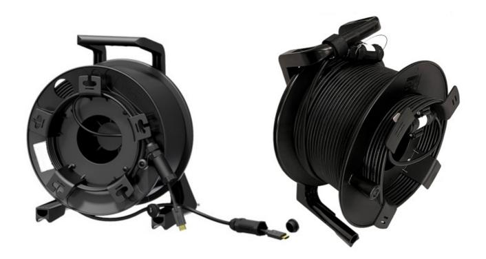
This rugged plastic unbreakable cable reel is environmental friendly and suitable for various types of long extension cables. The frame is made from a robust PC (Polycarbonate) integrated with handle and parking brake. The drum is made from special PE composite materials with detachable cable winder.
