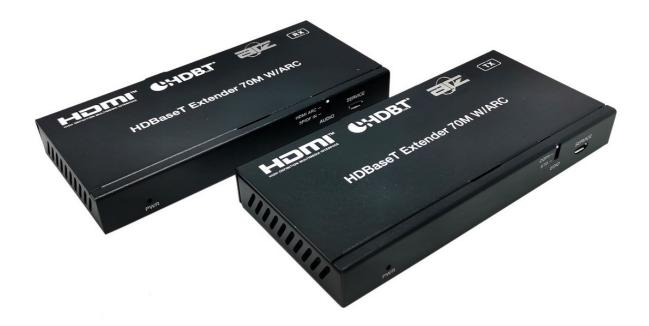
This 18Gbps HDBaseT Extender can extend HDMI signal, bi-directional IRcontrol signal, ARC signal and RS-232 control signal to a distance up to 70m / 230ft via a single CAT5e/6 cable. This product converts HDMI signal
