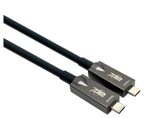
This is a FULL function USB type-C active optical cable (AOC) using optical fiber to replace copper wire as the high-speed signal transmission medium, it can perfectly transmit USB2.0, USB3.2 Gen2 and 2-lane DP1.4 data with excellent signal quality. Compared with the traditional copper wire, it is softer, slimmer, lighter and with perfect EMI/EMC feature. And it also has better reliability performance than copper wire.
