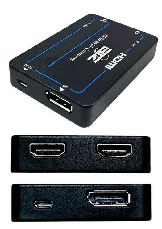
This HDMI to DP Converter has 1x HDMI INPUT, 1x HDMI LOOPOUT and 1x DP OUTPUT, which can convert HDMI signal to DP signal with video resolution up to 4K2K@60Hz 4:4:4. The DP port supports DP1.2.
