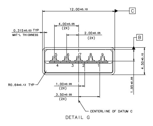
**USB 3.0 Standard-A Plug Pin Assignment**
