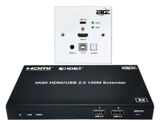
This 4K60 HDMI/USB-C 2x1 HDBT Wall-plate Transmitter support 1x HDMI input and 1x USB-C input within a standard 86mm×86mm wall box. It can transmit HDMI high-definition signal, bidirectional IR control signal, bidirectional RS-232 control signal and USB 2.0 signal over CAT6 to the distance up to 328ft/100m (HBT mode) or 492ft/150m (LRM mode). Video resolution is up to 4K2K@60Hz (4:4:4).
