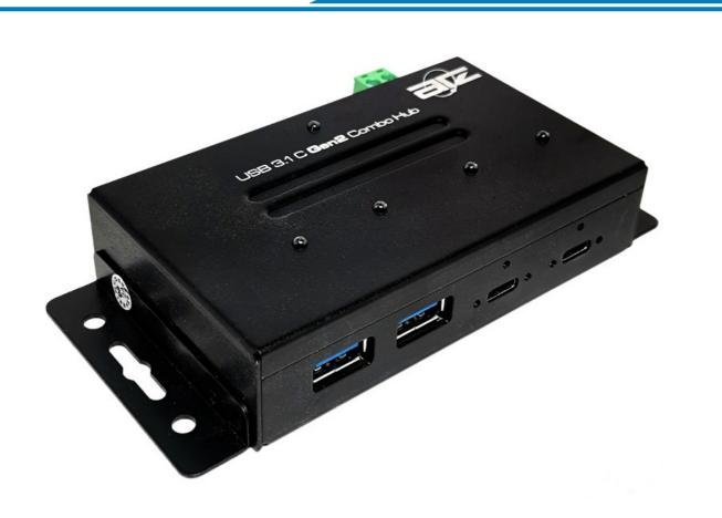
This ATZ UH304C-IND - provide 4-ports of additional 2x USB Type-A + 2x USB Type-C port to a USB C computer.
