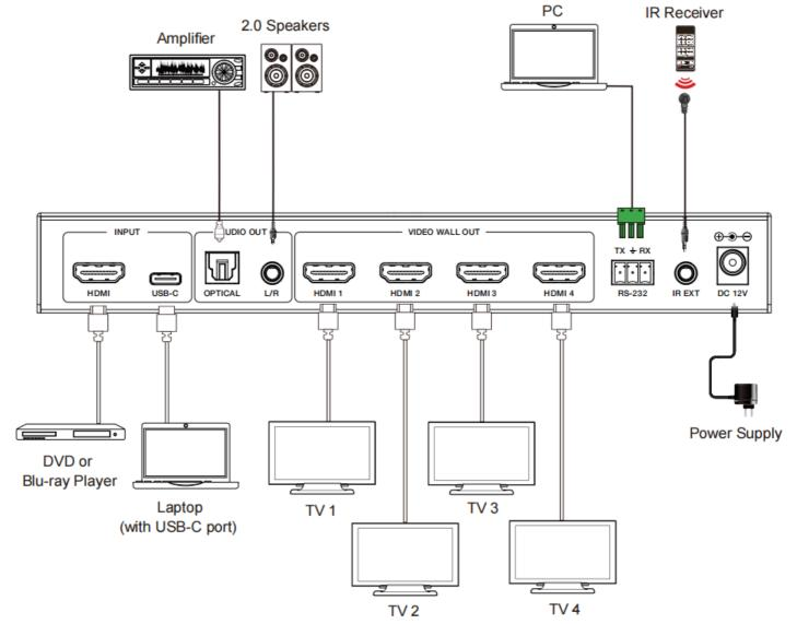
**Description:** 1x4 HDMI2.0 18G Video Wall Controller HDMI+USB-C input (2x2
