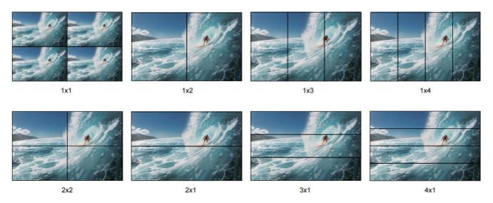
User can set display modes via front panel buttons, IR remote, and RS-232 commands.
