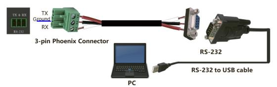
Then, open a Serial Command tool on PC to send ASCII command to control the device. The ASCII command list is shown as below.
