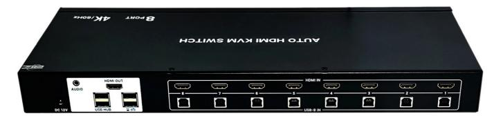
This KVM switcher can save you money, space, devices, and power consumption. It can control multiple computers through a set of keyboards, mouse, and displays. The KVM multi computer switch has features such as hot key switching, panel buttons, and automatic scanning.
