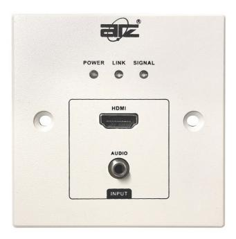
ATZ HDBT-E100-TW-A is a newly developed HDBaseT transmitter. It supports both input EDID management (with 7 built-in EDIDs), and external display's EDID. It supports 1080p60Hz up to 100m, 4K30Hz/ 4K60Hz(4:2:0) up to 70m over Cat5E/6 cable.
