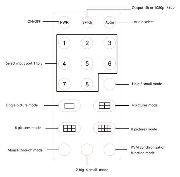
**Description:** 8-ports HDMI Quad Multi-viewer KVM Switch w/IR+USB (4K/30Hz
