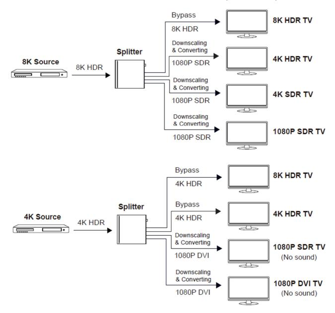
**Note:** If the source resolution is downscaled and converted to **1080P DVI** according to the EDID of display devices, it will be output without sound on TV.
