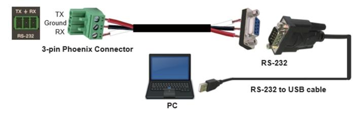
Then, open a Serial Command tool on PC to send ASCII commands to control the product. The ASCII commands list about the product is shown as below.
