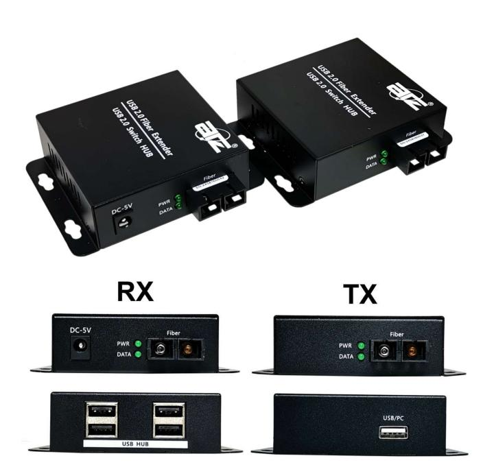
The USB 2.0 fiber extender transmits USB 2.0 signals at 480Mbps to 20KM through two or one optical fibers, and can also expand one USB 2.0 interface to four USB 2.0 interfaces. The USB 2.0 fiber extender consists of a transmitter and a receiver.
