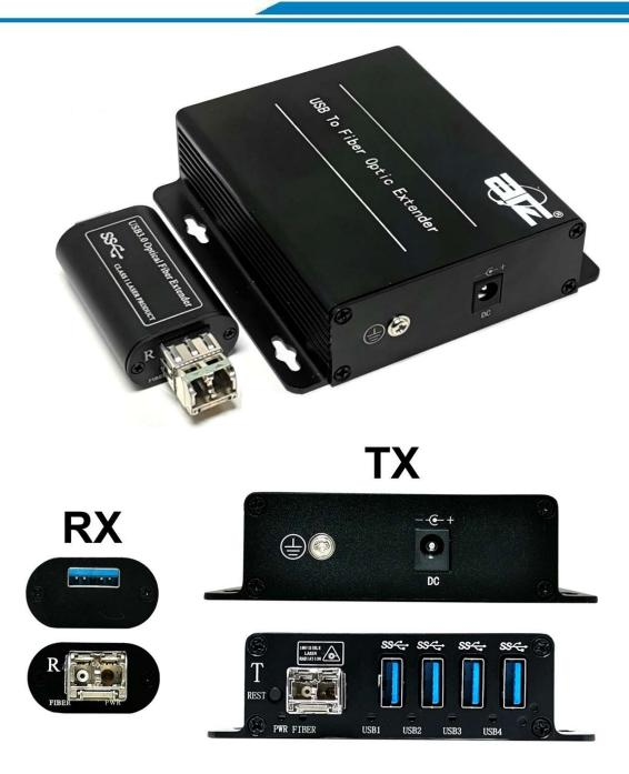
The USB 3.0 fiber extender transmits USB 3.0 signals at 5Gbps to 250 meters through two or one optical fibers, and can also expand one USB 3.0 interface to four USB 3.0 interfaces.
