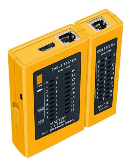
This ATZ NET-CBT02 is a high definition HDMI, RJ45 or RJ 11 cable tester. It is use to test each wire and cable pair individually, allowing for quick identification of correct and incorrect wiring configurations, detecting short circuits and open circuit. Allow testing of shielded network cable which is not available on most cable tester. Tester also provide intelligent detection with sequential LED indicator for accurate diagnostics.
