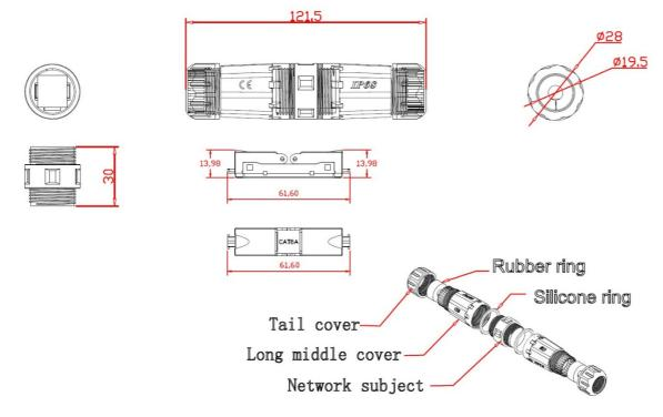
**Description:** IP68 Waterproof RJ45 Cat 6A / Cat 5 Inline Tool-less module Dual
